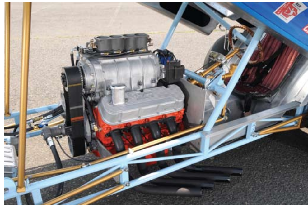
In 1969, a 427-cubic-inch Chevrolet (yes, Chevrolet) engine utilized a Hilborn injection system, Mallory ignition and a single fuel pump. Sanders said, "Chevy cars used Chevy engines, Fords used Fords and Chryslers used Chrysler. That's when you could recognize what the car actually was."
