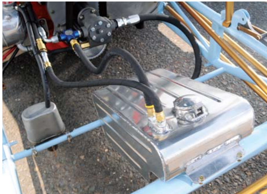
Jungle Jim had Al Bergler tool up these larger aluminum fuel tanks, which allowed both Jungle and Sanders to do those long smoky burnouts that the crowds loved.
