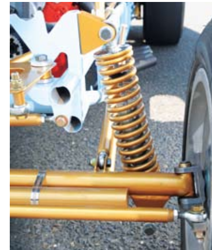
Yes, front suspension! Coil-over shocks allowed the cars a little bit of front end movement to help weight transfer.
